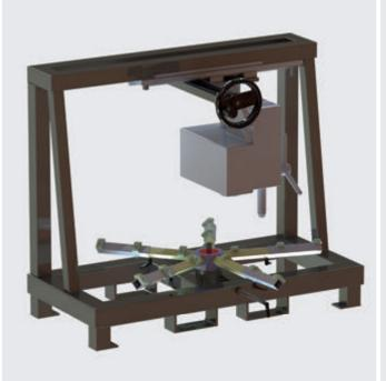
Drilling device for grinding wheels
