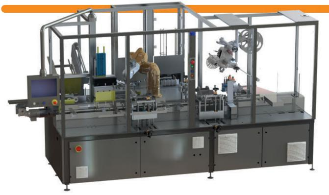
The 6-axis robot arm allows flexible solutions for packaging vials into folding card boxes including information leaflets and an optional cardboard separator..
